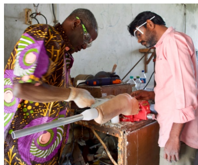
E.Kalanzi showing Jabbar how to build the positive mold of the Monolimb .
